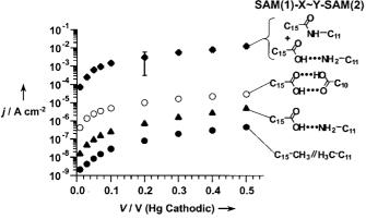
Figure 3. Plots of current density as a function of the bias voltage between the mercury and gold electrodes for  $J_{Au-SAM(1)-X\sim Y-SAM(2)-Hg}$ . The error bar is  $\pm$  the standard deviation of the data, s.
